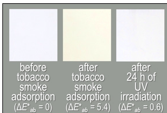
Figure 10. Photographs of the non-woven fabrics with TiO 2 before tobacco smoke adsorption, after tobacco smoke adsorption (0 h), and after 24 h of UV irradiation.
